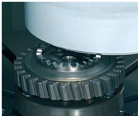
Curvic coupling face gear
